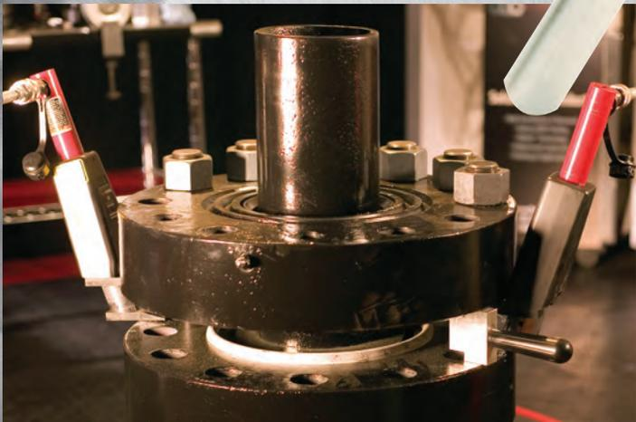
**Both manual and hydraulic AutoSPREADERs come complete with two safety blocks.**
