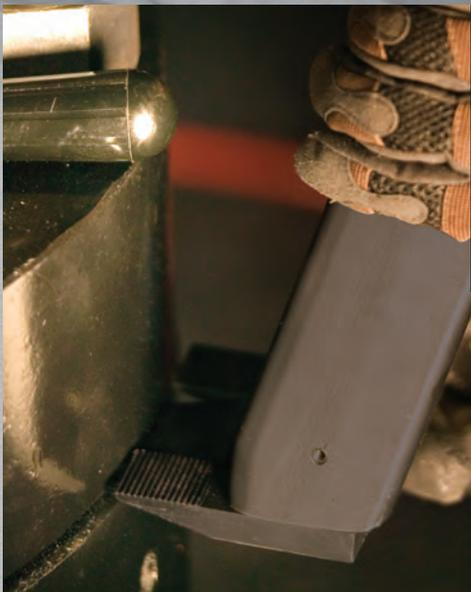
**The serrated feet on AutoSPREADER keeps it in place and only needs 3/32" of space to insert.**
