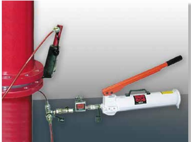
Hand Pump Model 100H2 is recommended to provide hydraulic power to a pair of HS10K AutoSPREADERS.
