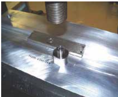
Figure 3. Galled Test Button and Block
