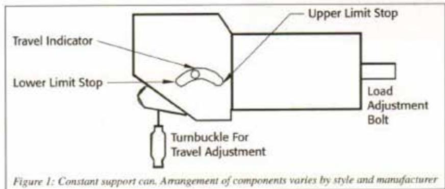
Figure 1: Constant support can. Arrangement of components varies by style and manufacturer
